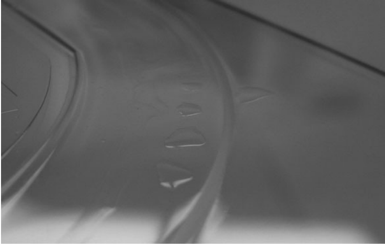
Fig. 4.45 Bubbles beginning to form due to high emboss temperature
