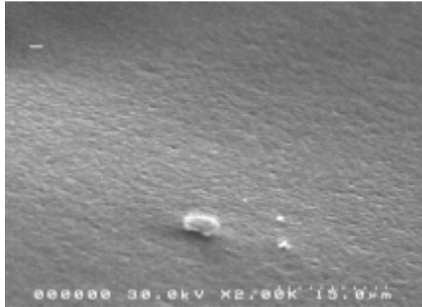
Fig. 7.3 Typical texture of the single-crystal silicon surface resulting after etching in \text{XeF}_2 gas phase etching
