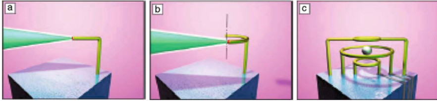
Fig. 9.39 Schematic illustration of LCVD process (Reprinted with permission from [136])
