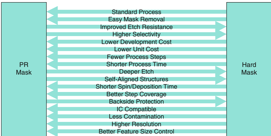
Fig. 8.6 Considerations and consequences of using a hard mask or a photoresist mask shows that a PR mask is generally the mask of choice, except for situations where higher etch resistance, a deeper etch, or substrate backside protection is needed
